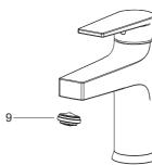
Ensure that all connections are tightened. Ensure that the handle is in the off position. Turn on the drain and main water supply, and check for leaks. Repair as needed.
