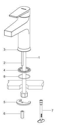
Install the mounting stud(2) onto the bottom(3) of the faucet.
